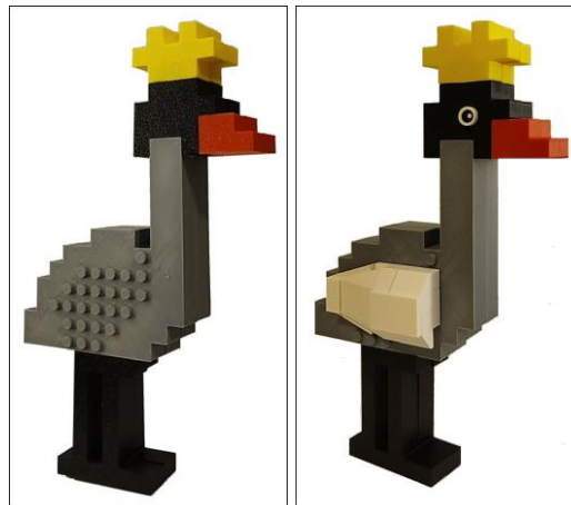
Figure 5.12. A printed framework with a skin of LEGO bricks applied over it.
