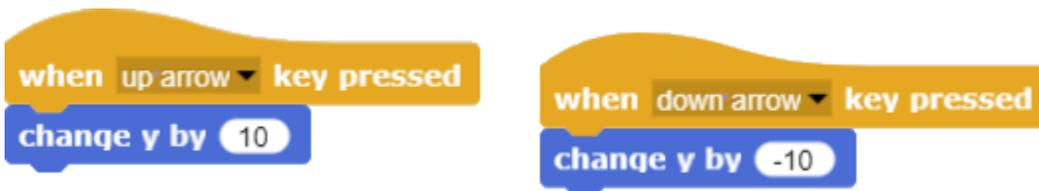
When the *up arrow* key is pressed, the **Change Y by 10** block is used to move the paddle upward. When the *down arrow* key is pressed, the **Change Y by -10** block is used to move the paddle downward.
