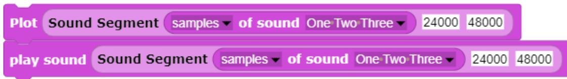
It may be more convenient to enter the start and end of the sound segment in milliseconds rather than in sound samples. This conversion can be accomplished by multiplying milliseconds by 48 (since 48 times 1000 milliseconds yields 48,000 sound samples). The addition of the label *Ms* after the input slots to indicate the units of measurement employed improves clarity.
