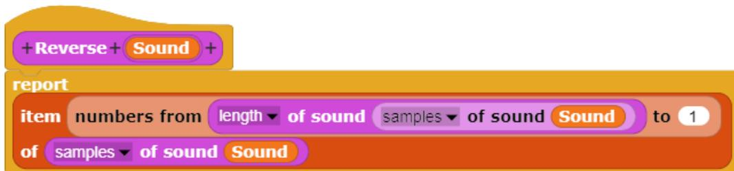
The **Reverse** code block reverses a sound, starting with the end of the list of sound samples and continuing to the first item in the list of sound samples.
