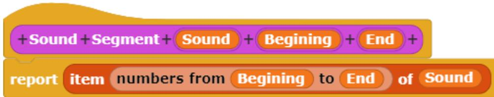
One benefit of creating a custom **Sound Segment** code block is that this code block can not only be used to graph a sound segment but also to play the sound segment to verify that the portion of the utterance obtained is the desired segment.
