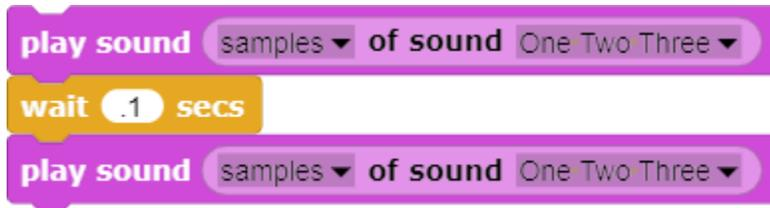
Musicians often use this method to create reverberation. A permanent list that combines one list of sound samples with a second, delayed list of samples can be created by placing a series of empty cells at the beginning of the second list. If the items from -10,000 to the **Length of the List** are displayed, the first 10,000 items in the list will be empty.
