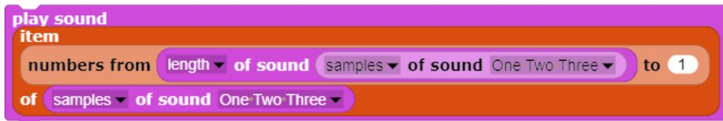
This method can be used to create a custom code block, **Reverse**, to reverse the sound.
