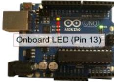
This LED can be used to test *Snap4Arduino* programs. Drag the Arduino code block Set Digital Pin \_\_\_ to \_\_\_ into the *Snap4Arduino* script area. Then drag the True / False code block (found under the *Operators* command palette) into the hexagonal slot at the end of the Set Digital Pin command.
