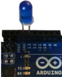
When Digital Pin 13 is turned on, both the onboard (yellow) LED and the external LED inserted into the pin socket will light up.
