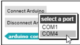
If the correct communications port is selected, the program will report, “An Arduino has been connected. Happy prototyping!”
