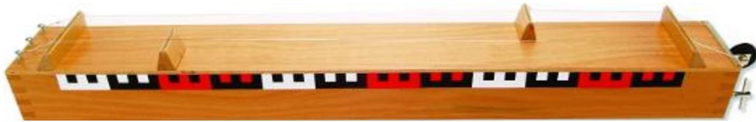
Figure 28. A monochord constructed with a guitar string.
