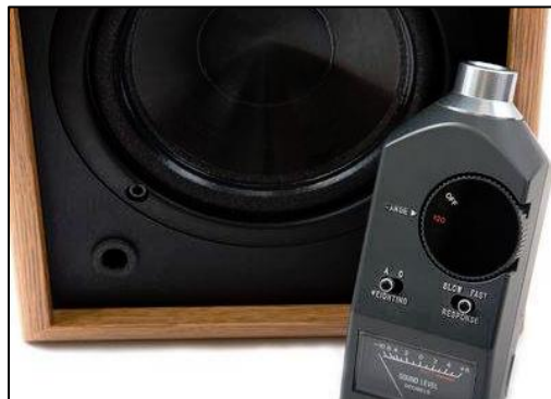
Figure 22. Measuring the intensity of a tone with a sound level meter.
