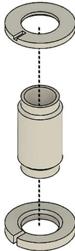
Glue the ring with the split in it to the closed end of the tube, as shown.
