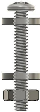
Put two washers and a nut on each screw as shown.
