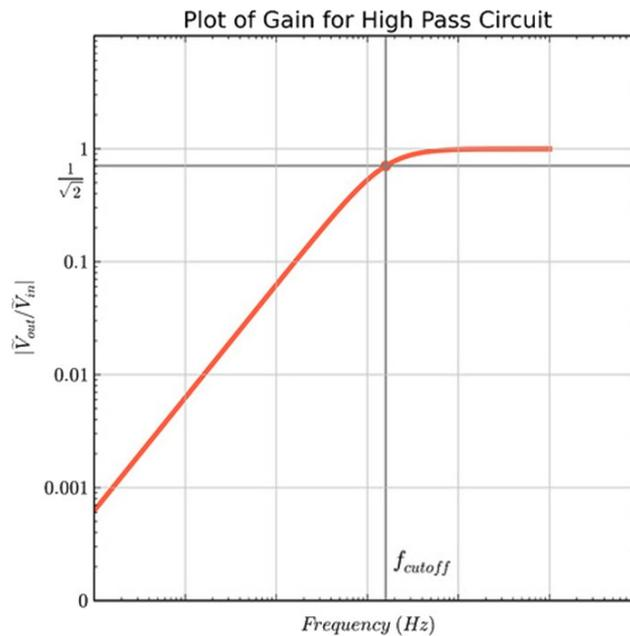
The controls on the Caustic SubSynth filter can be adjusted to create a cutoff frequency for three types of filters: a high-pass filter (that passes the higher frequencies), a low pass filter (that passes the lower frequencies), and a band pass filter (that passes frequencies in the middle of the spectrum).
